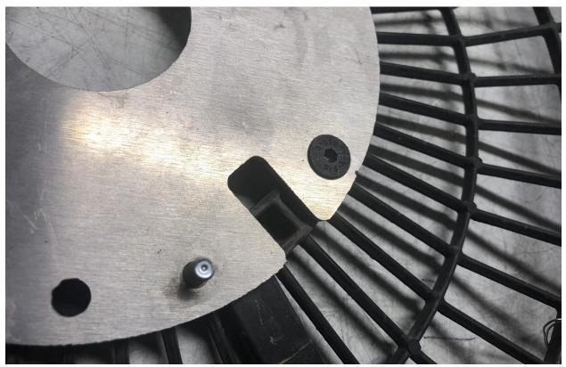
USE TAPERED BOLTS TO SECURE BRACKET – MAY HAVE TO DRILL WITH PILOT HOLE TO ENLARGE
