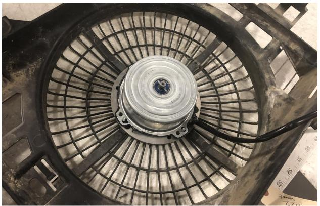
SET FAN MOTOR IN PLACE ON THE 4 MOUNTING STUDS – MAKE SURE BUMP ON FAN MOTOR SITS INTO THE CUTOUT ON THE BRACKET (SEE BRACKET CUTOUT ON PREVIOUS PICTURE)
