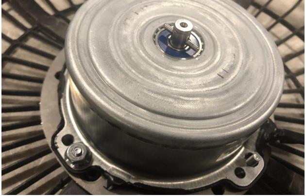
USE NUTS TO SECURE FAN MOTOR TO THE BRACKET AND INSERT PIN IN MOTOR SHAFT
