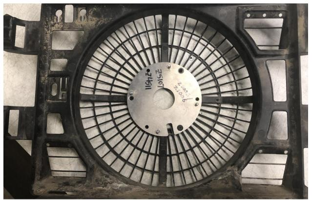
SET BRACKET ON THE FAN BLADE SIDE OF THE SHROUGH - ALIGN WITH THE 3 MOUNTING HOLES
