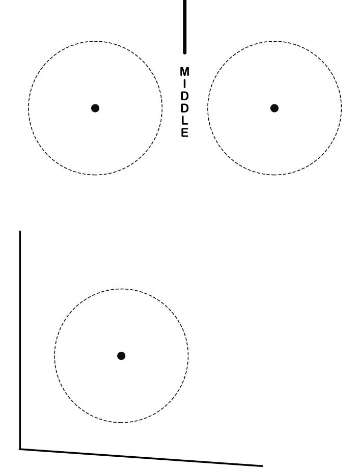
Cut Out Templates are size of the louver face (NOT hole-saw cut-out). Use this to mark the spot to start the hole-saw bit.
