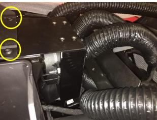
The heater is mounted in the middle of the dash, between two cross bars with the fittings facing the driver side. There are two factory bolts that are used to mount the heater bracket. When setting the heater in place it is going to be a tight fit. Run the attached hoses down towards the driver side floor and you are going to have to put some force against the two bottom duct hoses to get the heater in place (it is perfectly OK to scrunch the duct runs a little). See mount pic below:
