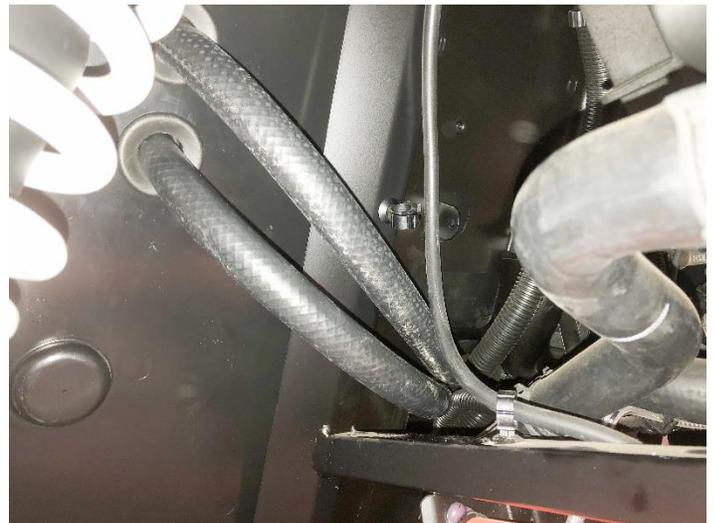
Run the two 6.5-foot runs of heater hose from the core fittings, through the grommets and then run them alongside the radiator lines to the back of the machine (engine) as shown below. Use a couple zip ties to secure the heater hose to the steel radiator lines.
