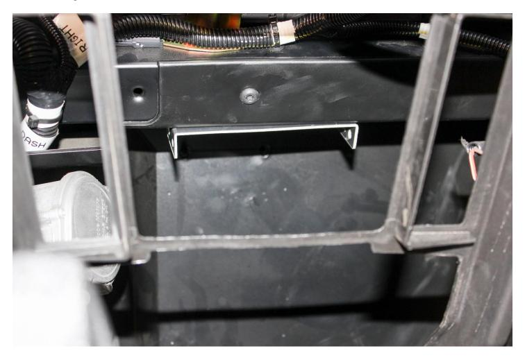
Once the top mounting place is secured to the framing, you can then mount the heater box bracket to it. This will require a 3/8 socket to secure the 4 bolts from the sides. Mount the heater so that the duct holes are facing towards the rear of the machine and the core fittings are pointed toward the passenger side, as shown below.
