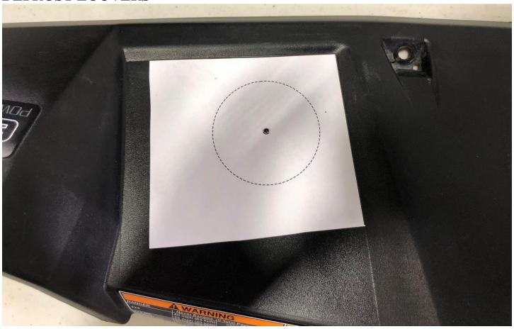
Now with your two defrost louvers installed in the top dash panel you can move onto the floor louvers. To start you are going to cut open the center cubby hole as shown below. There is no exact way to cut this opening out, we drilled 4 holes with a ½" drill bit and then make cuts connecting them. You could also use a large hole-saw (3+ inches) and create a good access cut-out for this step. See the photo below for how we did it.
