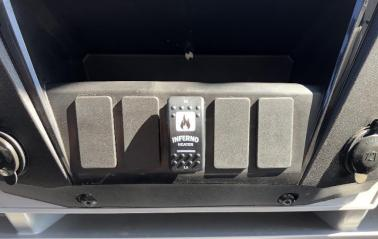
The 12v power wire is shown below. The Red and the Black connectors need to be plugged into the back of the switch as shown on the previous page and the OE 12v connector plugs into one of the open power sources located behind the dash (see picture below). At this time, make sure the heater system runs correctly. We will move on to final install and replacing the machine panels soon.
