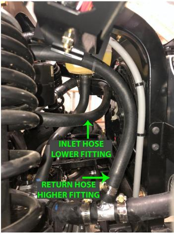
RETURN LINE FITTING (CONNECT TO HIGHEST CORE FITTING RELATIVE TO GRAVITY)
