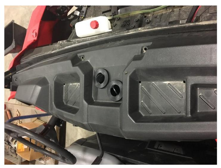
Now with your two defrost louvers installed in the top dash panel you can move onto the floor louvers. To start you are going to cut open the center cubby hole as shown below. There is no exact way to cut this opening out, we drilled 4 holes with a ½" drill bit and then make cuts connecting them. You could also use a large hole-saw (3+ inches) and create a good access cut-out for this step. See the photo below for how we did it.
