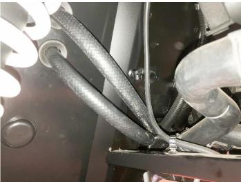
14-feet of heater hose is provided in the kit, cut this into 87" (inlet) and 81" (return) hose pieces. You will run your heater hose from the heater box to the back of the machine where we will splice into the coolant lines. Start by running your heater hose from the front of the machine, down under skid plate. With the seat and the
