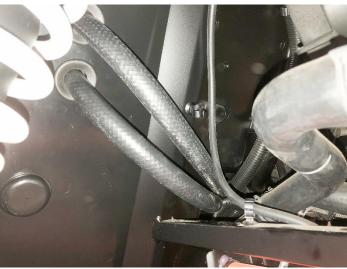
Run the two 6.5-foot runs of heater hose from the core fittings, through the grommets and then run them alongside the radiator lines to the back of the machine (engine) as shown below. Use a couple zip ties to secure the heater hose to the steel radiator lines.
