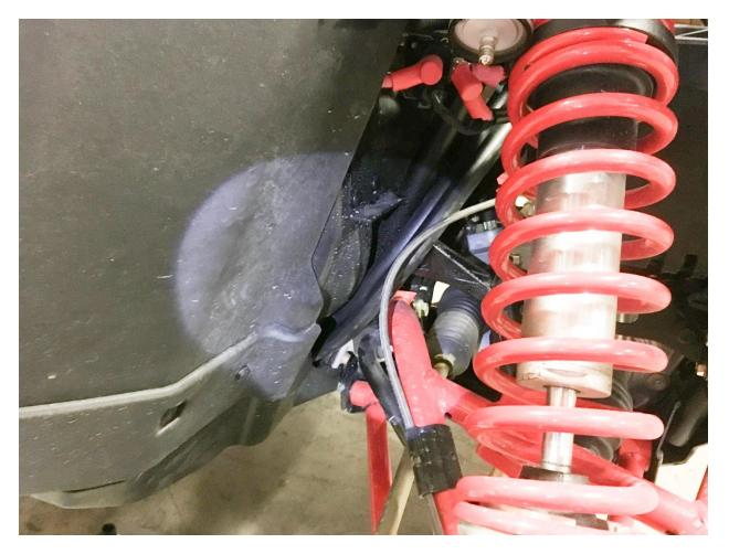
Once you have the heater hose fed to the back of the machine you can install your Y-Fittings. Your inlet line will splice into the upper radiator line, this will connect with the lower heater core fitting (relative to gravity). Conversely, the lower radiator line will connect with the higher heater core fitting (relative to gravity). If you do not have hose clamps to use when installing the Y-Fittings, drain the radiator prior to cutting into the radiator hose.
