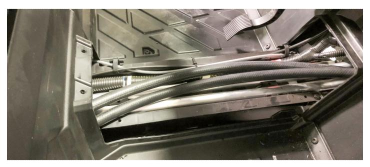
Now locate the factory plastic 'T' under the seats and replace this with the Y-Fitting included in the kit (see photo below). Make sure the 5/8" splice off this Y-fitting is pointing towards the radiator, you want this coolant to flow back inline. See photo below where the plastic 'T' has been replaced with the Y-Fitting:
