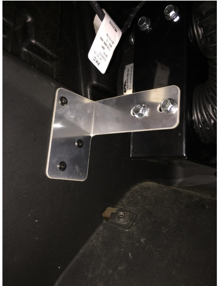
PICTURE TAKEN FROM DRIVER SEAT, TO THE LEFT OF THE STEERING WHEEL. REMOVE THE SMALL CUBBY FOR BETTER ACCESS.
