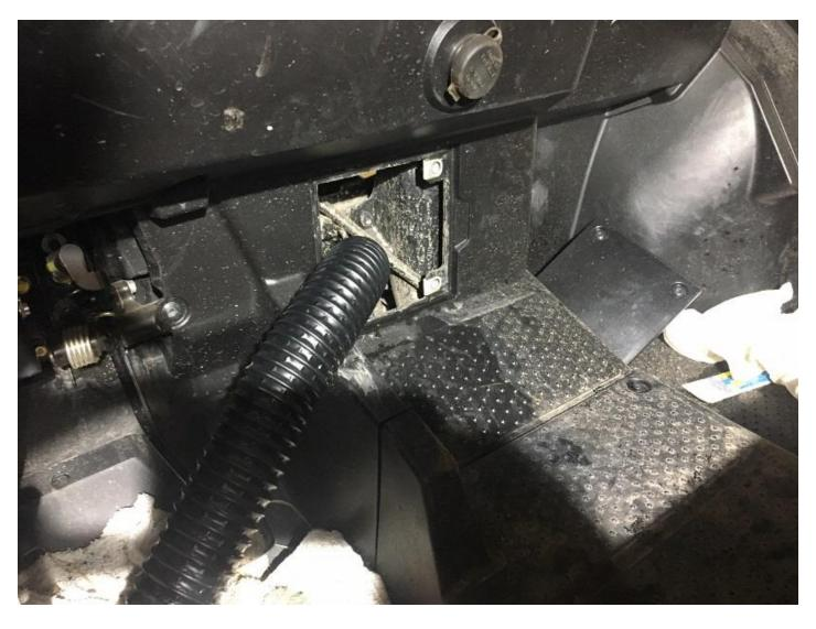
The two floor louvers were put in the locations below. Cut the remaining duct in half (roughly two 4-foot pieces will be left) and secure these pieces to the backs of the floor louvers. Bear down with the zip ties and run the duct toward the heater. Now attach the 3 runs of duct to the heater and clamp down with zip ties. You are now done with the duct work.
