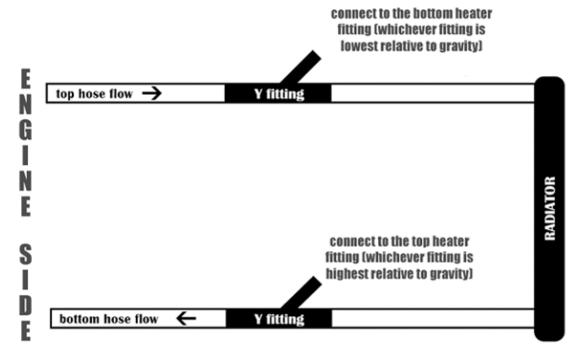
The easiest place to splice into the radiator hose is underneath the middle seat (See Photo below). Cut into the radiator lines and install the Y-Fittings, secure with the hose clamps provided. Run the heater hose from the Y-Fitting in the upper radiator hose to the heater core fitting that is lowest, relative to gravity. Run the other hose from the lower (Return Line) radiator hose to the heater core fitting that is highest relative to gravity.
