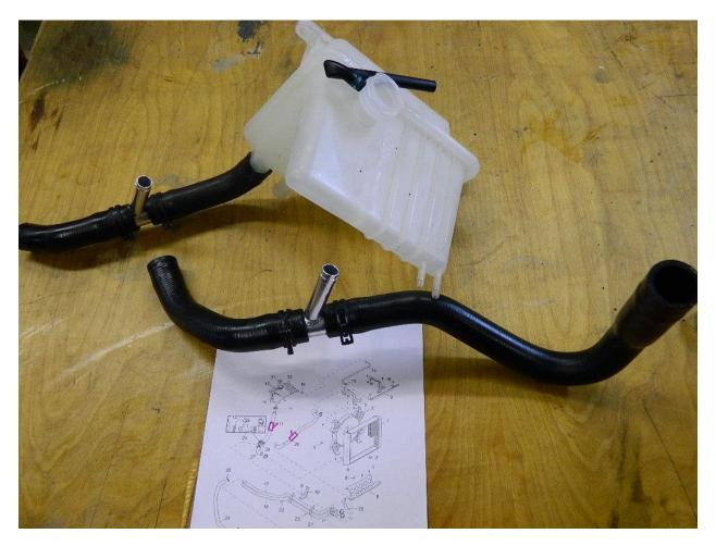
The splices need to be pointing towards the radiator because we want the coolant to flow easily to the heater (from the engine) and flow easily back into the radiator (engine) return hose. You will want to connect the "inlet line" heater hose to the lowest heater core fitting relative to gravity. The "return line" heater hose you will want to connect to the highest heater core fitting relative to gravity. See the diagram on the next page for further reference.
