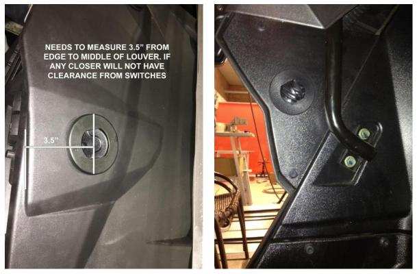
Last, attach the duct hose to the louvers and secure with the zip ties provided. Make sure you use a needle nose pliers and bear down on the zip-tie to insure a tight hold. Then run the hose up to the heater and secure with a zip tie to the heater box duct adapters. After all four louvers are attached you can reattach your dash panel and fenders.
