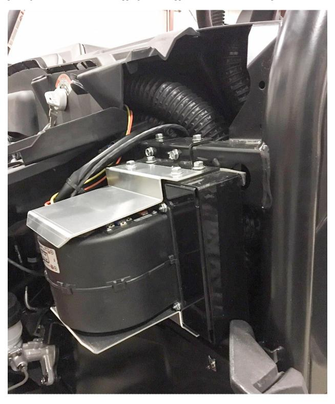
After you mount the heater you can attach the heater hose from the Y-Fitting splices to the heater core fittings. Run the heater hose from the Y-Fitting in the upper radiator hose to the heater core fitting that is lower than the other fitting (relative to gravity). Run the other hose from the lower radiator hose to the higher heater core fitting (relative to gravity). See diagram below:
