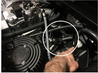
Now you can attach the heater hose to the 5/8" y-fitting splices. Run the heater hose from the y-fitting in the upper radiator hose to the heater core outlet (outlet is the fitting that is lower than the other fitting). Run the other hose from the lower radiator hose to the heater core inlet fitting. We include enough heater hose so you have room to slowly turn the hose into the heater ports to avoid kinking the hoses.
